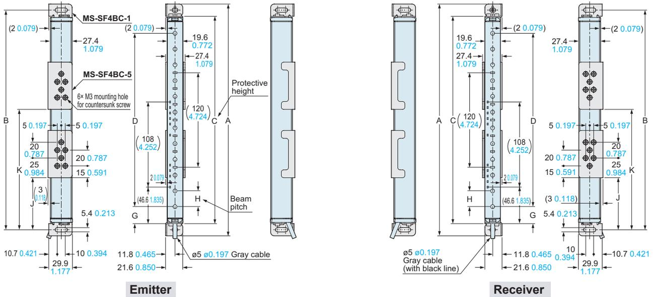
**<Connector of the pigtailed type (with muting function) SF4B-□CA-J05>**
