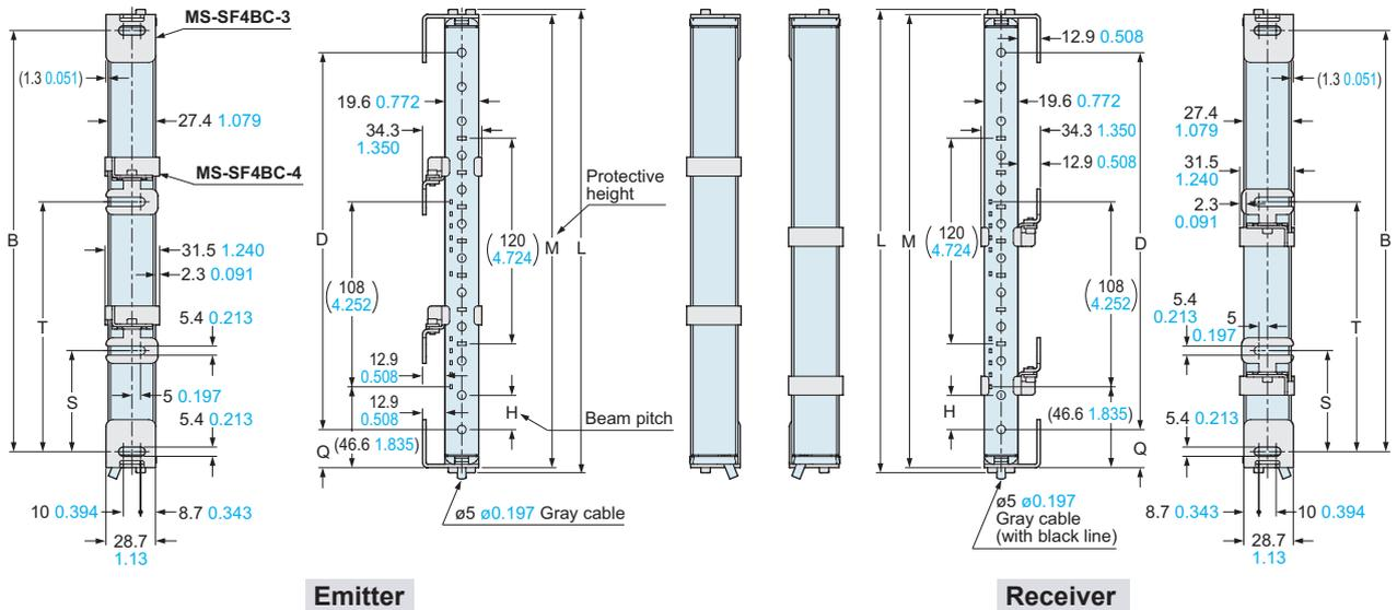
**<Connector of the pigtailed type (with muting function) SF4B-□CA-J05>**
